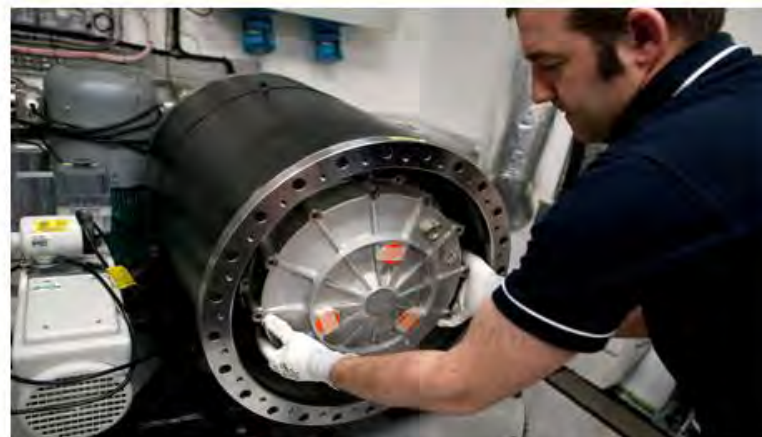
Part of the flywheel energy storage system at Williams's factory in Wantage. Photograph: Simon Dawson/Getty Images
